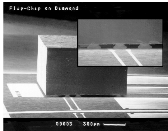
Fig. 8 a) Diamond flip-chip mount using CPW technology with 28GHz GaAs PHEMT power amplifier MMIC. b) mounted amplifier MMIC using ball bond technology
